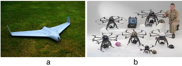
**Gambar 1.** Drone a) *fixed wing*, b) *rotary wing*
